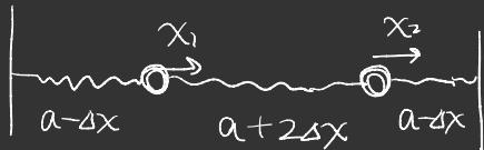
$$m \ddot{x}_1 = k \cdot (2\Delta x + x_2 - x_1) + k(x_1 - x_0) - \frac{k e q^2}{(a + 2\Delta x + x_1 - x_2)^2}$$
