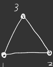
(a) In 2D motion, each mass has 2 degrees of freedom. There could be 6 normal modes however, due to the restrictions in the 3 force connections between them, there should be 3 zero modes.
