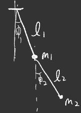
$$L = \frac{1}{2} m_1 l_1^2 \dot{\phi}_1^2 + \frac{1}{2} m_2 (l_1^2 \dot{\phi}_1^2 + l_2^2 \dot{\phi}_2^2 + 2 l_1 l_2 \cos(\phi_1 - \phi_2) \dot{\phi}_1 \dot{\phi}_2)$$
