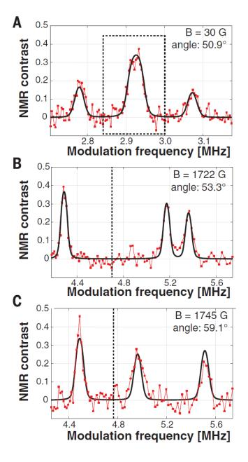
Satellite peaks: dipole-forbidden transitions become weakly allowed due to mixing by the **B** component perpendicular to the h-BN principal axis
