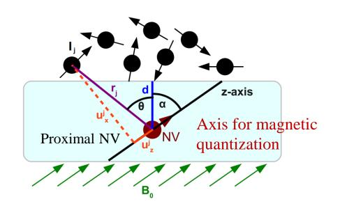
Measure statistical fluctuations of the spin polarization  $\sim \sqrt{N}$  (independent of the applied field)
